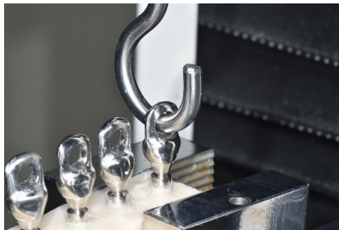
Fig. 6. Evaluation of retentive force measurement by the universal testing machine (TW-D102; Taewon Tech Co.).
